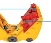
Interchangeable teeth mounted on a bolt-on plate with tooth sockets
