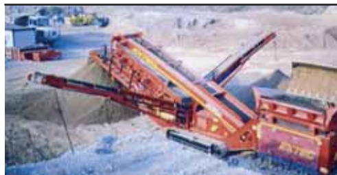
Dual mobile Extec S-4 screening plant for reclaiming an abandoned industrial site in Milan.
